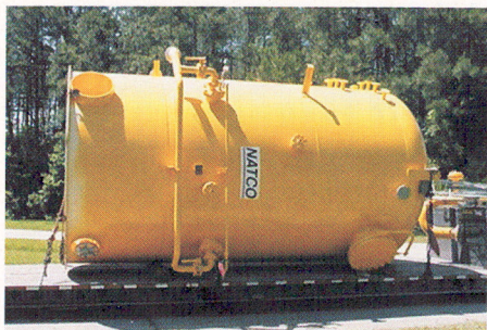
Figure 1. Photo of a VersaFlo unit (capacity of 6,400 m 3 /day) ready to be shipped to a deep water platform in The Gulf of Mexico.
