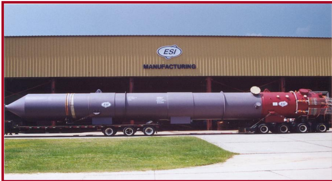
Fig. 8—A vertical submerged column flotation unit with a capacity to process 115,000 BWPD is shown ready for shipment to be installed on a deep-water spar-type platform.
