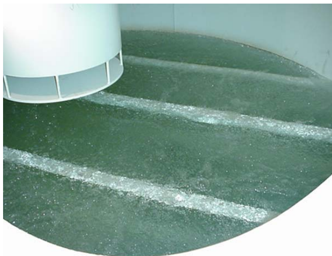
Fig. 3. Four radial eductors distribute flotation bubbles over the cross sectional area of a 10 ft. diameter VersaFlo™. The water discharge end of the cyclonic inlet is also visible.
