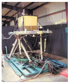
Separating oil, water, and gas is particularly difficult on floating platforms because wave motion tends to mix the three phases. Natco previously relied on costly physical testing to evaluate separator designs. This did not allow the visualization of the liquid phase movement inside the vessel. Using computational fluid dynamics (CFD) software to study the hydrodynamics inside a separator, engineers can see what happens to the oil, water, and gas during even the most complicated wave motions.
