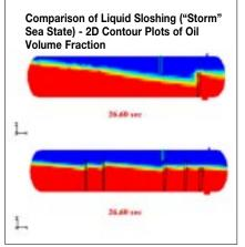
with FLUENT's postprocessor, made it easy to see the severe sloshing inside the vessel. Next he modelled the separator with baffles, which were specified as porous media, in the vertical orientation, trying different baffle materials, shapes, and degrees of porosity. He ran multiple CFD analyses to find the most effective
