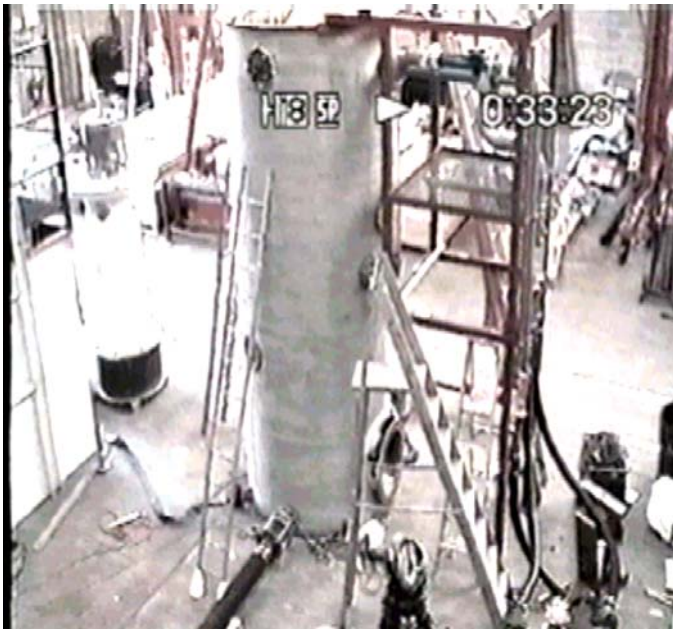
Fig. 2. The 5-ft diameter by 15-ft tall tank at the NATCO-Axsia facility in Gloucester, U. K. that was used to validate and extend the results of CFD simulations for the vertical column flotation technology development program.
