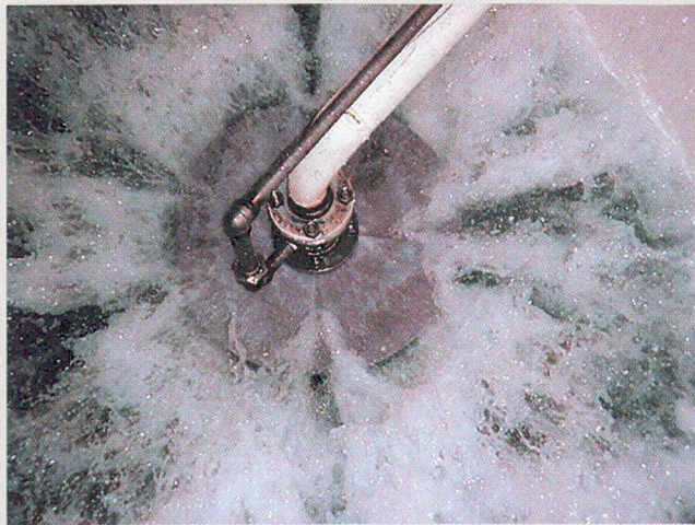
Fig. 6. Radial eductor installed in a 40,000-bwpd VCF.
