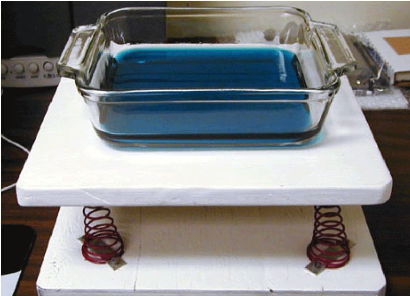
Close-Up of Rocking Table Model
