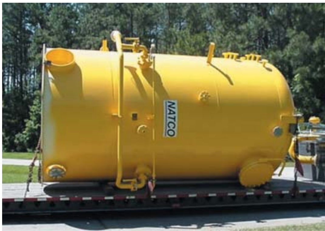
Figure 1: Photo of a VersaFlo™ unit (capacity of 6,400 m 3 /day) ready to be shipped to a deep water platform in The Gulf of Mexico
